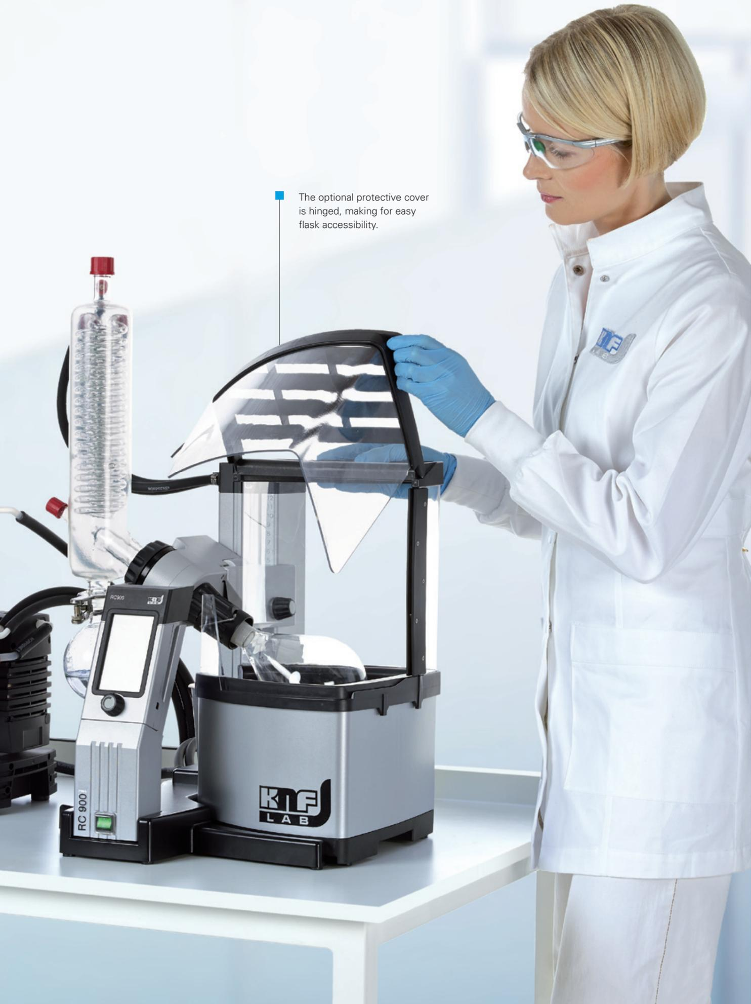
■ The optional protective cover is hinged, making for easy flask accessibility.
